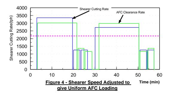
It is interesting to note that a significant reason for the overall inefficiency of the Full Web Bi-Di Cutting Cycle, is that the shearer spends a significant portion of its time in unproductive maneuvers at the ends of the runs. These have a greater effect on narrower faces, but are still important on even very wide faces.
