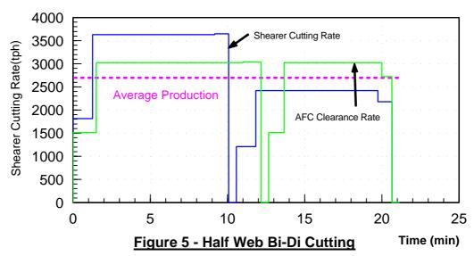
For the same overall production rate, a Half Web approach requires much higher shearer speeds than a Full Web cycle. This is because in a single up and back pass, the shearer will only cut one drum width, while with the Full Web cycle, two drum widths are cut. However the Half Web option does have some significant benefits.
