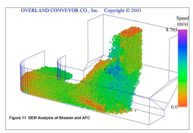
The latest research in this field is looking at modeling the actual longwall operation, including the Shearer and AFC. Currently little or no science is used in the design and analysis of these components. With the ability to visualise the mechanics of these elements in operation, it is expected that better designs will be forthcoming. Figure 11 shows a simple model of a shearer and AFC in operation.
