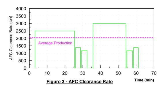
If a cutting cycle such as this is used, while the shearer needs to be sized at only 2750tph, the AFC and conveyors must be sized for 3000tph and the average production for a perfect cycle is only 2000tph.
