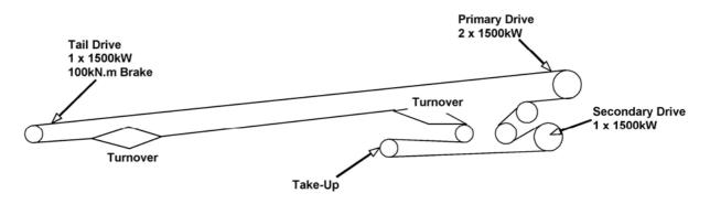
Figure 2. Layout of Tianjin Coal Transport Conveyor
