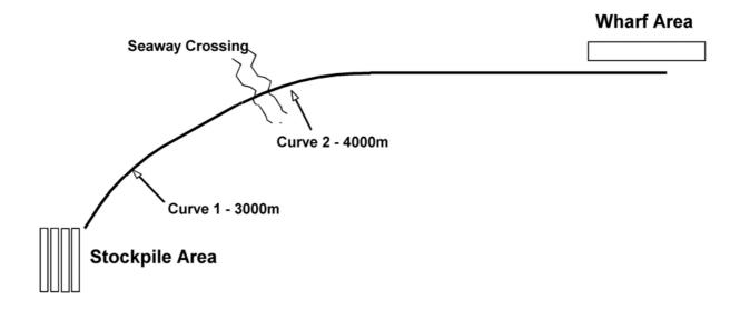
Figure 1. Route for Tianjin Coal Transport Conveyor
