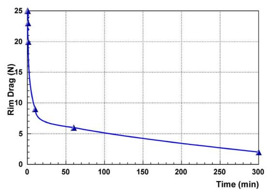
Figure 4. Tianjin Coal Conveyor – Carry Roll Rim Drag Measurements
